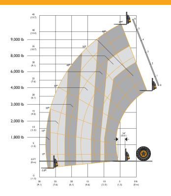
This load chart is for the rated capacity of the machine with 66" wide standard carriage and 48" pallet forks. Use only JCB approved attachments and check the relevant load chart for the machine model. If in doubt, consult your dealer. If the load rating of the machine differs to that of the attachment, the lower rating becomes the overall capacity. Automatic rear axle stabilization (RAS) system.
